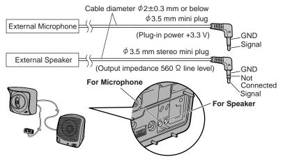
• The external microphone input terminal does not correspond to an line level. Audio may be distorted when the line level is input. Audio distortion will be solved if you insert the following circuits. Under no circumstance should high level audio, such as from a speaker, be connected to this input terminal. Doing so is likely to damage the camera.
