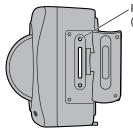
RESTART Button (Press the button with a pointed object.)
